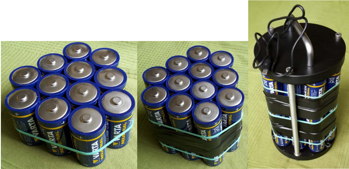
Figure 3: Filling the battery canister. It is advised to apply tape around every single layer as well (not shown here) for larger stability of the battery pack.
